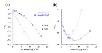
Fig. 4 Stability of unencapsulated receptor/CNT and Li<sup>+</sup>-receptor/CNT in air at 373 K. (a) n-type seebeck coefficient to the initial n-type seebeck coefficient ( $S/S_0$ ), and (b) electrical conductivity to the initial electrical conductivity ( $\sigma/\sigma_0$ ) over duration.
