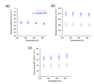
Fig. 2 (a) Seebeck coefficient, (b) electrical conductivity, and (c) power factor of the receptor/carbon nanotube (CNT) (pink) and Li+receptor/CNT (blue) plotted against temperature.
