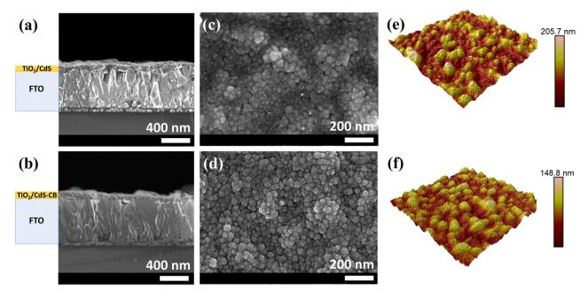
Fig. 3 SEM images showing the: (a and b) cross-sectional and (c and d) top views of TiO<sub>2</sub>/CdS and TiO<sub>2</sub>/CdS-CB substrates. (e and f) Surface AFM images of both substrates.
