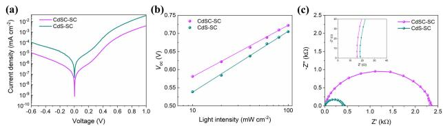
Fig. 6 (a) Dark J-V curves, (b)  $V_{oc}$  as a function of light intensity, and (c) Nyquist plots of CdSC-SC and CdS-SC devices. The inset of (c) shows a zoom-in of the high-frequency region.
