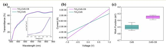
Fig. 4 (a) UV-vis transmittance spectra, (b) current-voltage curves, and (c) average work functions of the TiO<sub>2</sub>/CdS and TiO<sub>2</sub>/CdS-CB substrates. Inset in (a) shows the Tauc plot.
