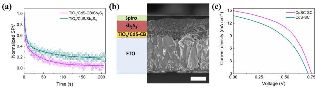
Fig. 5 (a) SPV decays of Sb<sub>2</sub>S<sub>3</sub> on TiO<sub>2</sub>/CdS and TiO<sub>2</sub>/CdS-CB substrates. (b) Cross-view SEM image of CdSC-SC. Inset bar: 200 nm. (c) J-V characteristics of the champion CdS-SC and CdSC-SC devices.
