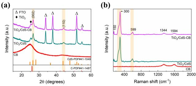
Fig. 1 (a) XRD patterns and (b) Raman spectra of CdS and CdS-CB films. The respective analysis of CB powders is also included. The orange regions correspond to the peaks related to CdS.
