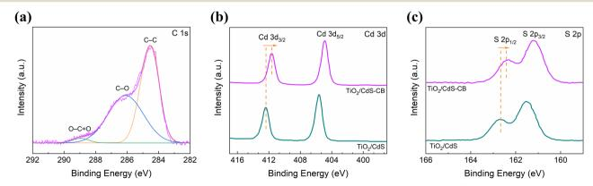
Fig. 2 (a) C 1s XPS spectrum of the CdS-CB nanocomposite film. (b) Cd 3d and (c) S 2p XPS spectra of the TiO<sub>2</sub>/CdS and TiO<sub>2</sub>/CdS-CB samples.
