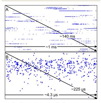
Fig. 2 Simplified visualization of spICP-MS data of a dispersion of 41 nm AuNP with nanosecond time resolution with a binary viewer program. (A) Several ion cloud signals during  $\sim\!\!140$  ms of acquisition. (B) Detector events in one individual ion cloud during  $\sim\!\!225~\mu s$  data acquisition. Note: each blue logical pixel represents a byte with a value unequal to 0 (1 or more DE), each white logical pixel represents a byte with the value 0 (no DE).
