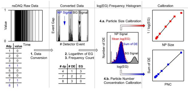
Fig. 9 Workflow diagram for the processing of nanosecond time-resolved spICP-MS data.
