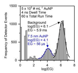
Fig. 5 Histogram of the frequency of detector events vs. the logarithm of the event gap (log(EG)). In the bimodal distribution, the right peak with longer event gaps between detector events (avrg.  $\sim\!5.9$  ms) corresponds to the background (black) while the left shoulder with a shorter mean event gap ( $\sim\!56~\mu s$ ) corresponds to ions from 7.5 nm AuNP (blue).
