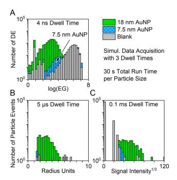
Fig. 8 Comparison of spICP-MS data acquired simultaneously with (A) 4 ns (nanoDAQ), (B) 5  $\mu s$  ( $\mu sDAQ$ ), and (C) 0.1 ms (vendor software) dwell time. Dispersions of AuNP with nominal sizes of 18 and 7.5 nm and a blank solution were measured for 30 s, respectively. Please note that the background signal of nanoDAQ data is on the right side (high log(EG)), while the background in plots from conventional spICP-MS is on the left.
