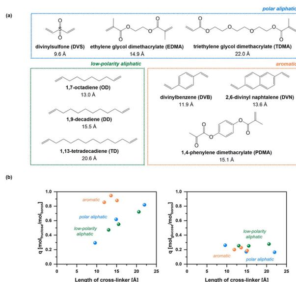
**Fig. 8** (a) Structures of the cross-linkers used to synthesize gel-type polymers with boronate moieties and (b) dependency of loadings of D-fructose (left) and D-glucose (right) on the nature of the cross-linker. This figure has been adapted from ref. 58 with permission from the Royal Society of Chemistry, copyright 2020.
