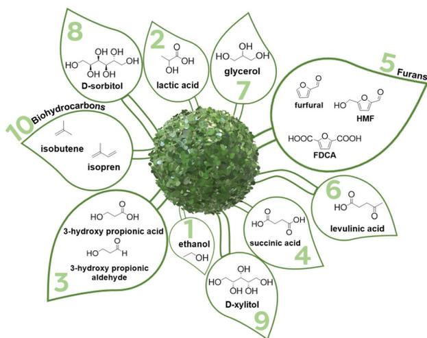
Fig. 1 Structures of ten molecules indicated by DoE as platform chemicals.<sup>5</sup>
