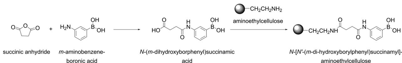
**Fig. 13** Two different routes for the grafting of boronic acid onto cellulose proposed by Weith *et al.* This figure has been reproduced from ref. 55 with permission from the American Chemical Society, copyright 1970.
