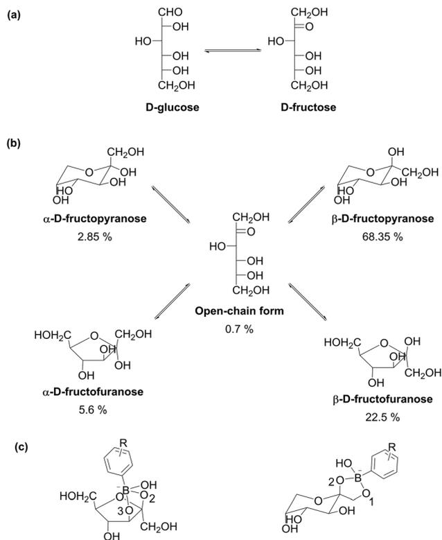
**Fig. 5** (a) Isomerization of  $\text{D-glucose}$  into  $\text{D-fructose}$ ; (b) equilibrium forms of  $[2-^{13}\text{C}]\text{-D-fructose}$  determined by  $^{13}\text{C}$  NMR at 25 °C in  $\text{D}_2\text{O}$  as solvent;<sup>70</sup> (c) complexes between boronate anions and anomers of  $\text{D-fructose}$ .<sup>62</sup>
