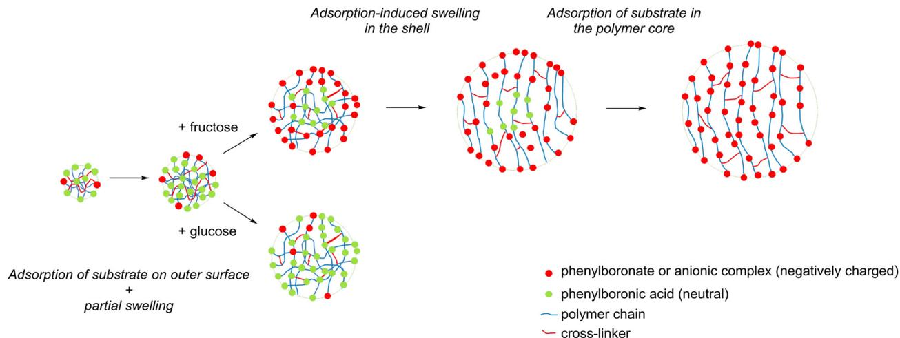
**Fig. 9** Scheme of swelling upon adsorption of D-fructose and D-glucose. This figure has been adapted from ref. 58 with permission from the Royal Society of Chemistry, copyright 2020.
