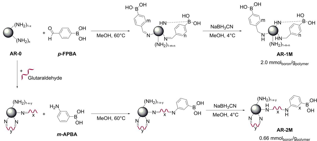
**Fig. 14** Synthetic routes for grafting phenylboronic acid moieties onto an amino microporous resin proposed by Wang *et al.* This figure has been reproduced from ref. 79 with permission from the American Chemical Society, copyright 2018. Abbreviations: aminated macroporous poly(styrene-co-divinylbenzene) resin (AR-0), *p*-formylphenylboronic acid (*p*-FPBA), 3-aminophenylboronic acid (*m*-APBA).
