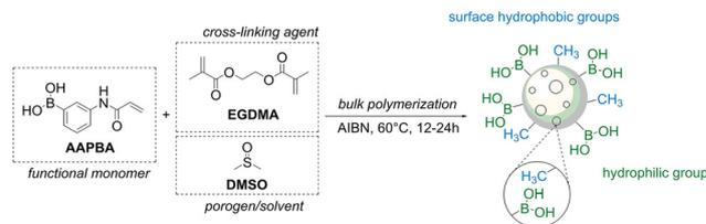
**Fig. 10** A method to produce a macroporous resin bearing boronic acid groups developed by Wang *et al.* This figure has been reproduced from ref. 76 with permission from the Elsevier, copyright 2019. Abbreviations: 3-acrylamidophenylboronic acid (AAPBA), ethylene glycol dimethylacrylate (EGMA), and dimethylsulfoxide (DMSO).
