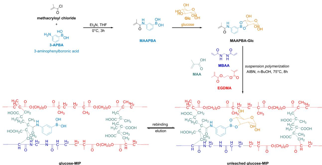
**Fig. 12** Molecularly imprinted polymer for a selective capture of D-glucose from cellulose hydrolysates. This figure has been reproduced from ref. 77 with permission from the John Wiley and Sons, copyright 2022. Abbreviations: 3-acrylamidophenylboronic acid (AAPBA), methacrylic acid (MAA), *N,N'*-methylenebisacrylamide (MBAA), ethylene glycol dimethylacrylate (EGMA), azobisisobutyronitrile (AIBN).
