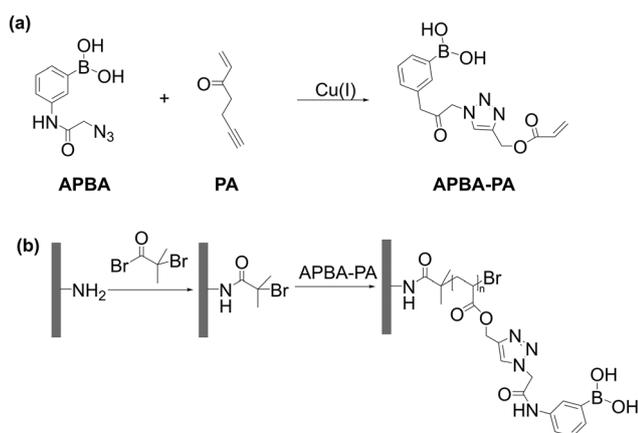
**Fig. 18** (a) Synthesis of boronic acid monomer and (b) its polymerization using surface-initiated ATRP. Reproduced with permission from ref. 83. Abbreviations: 3-(2-azido-acetylamino)phenylboronic acid (APBA) and propargyl acrylate (PA).
