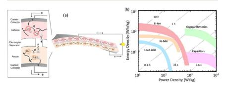
Fig. 2 (a) An organic, flexible paper-like battery fabricated using a pair of redox polymers and an electrolyte-containing thin-film separator and (b) batteries and capacitors plotted in a diagram of energy density vs. power density: Ragone plots (the h and s values represent the time required for full charging/discharging). (a) Reproduced from ref. 11b from the Royal Society of Chemistry 2022.
