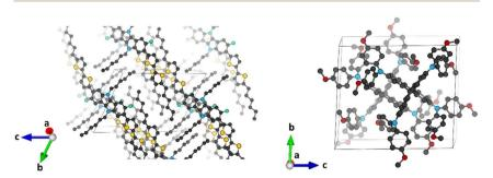
Fig. 2 Minimum-energy crystal structure calculated at the PBEsol level of theory for IDIDF (left) and spiro-OMeTAD (right). Color coding: C in black, S in yellow, N in blue, O in red and F in cyan. H atoms are omitted for clarity.
