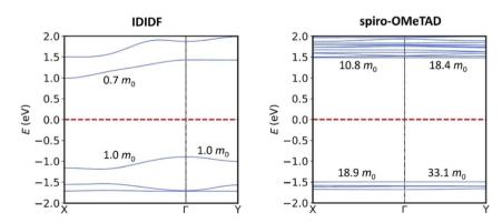
Fig. 3 Band structure calculated at the HSE06 level for IDIDF (left) and spiro-OMeTAD (right) on the PBEsol-optimized crystal geometries. Only two k-segments are displayed for simplicity (see Fig. S1† for full band structure diagrams). Relevant effective masses for holes (in the VBM) and for electrons (in the CBM) are indicated.
