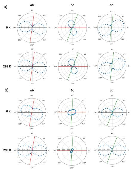
Fig. 7 Anisotropic plots of the hole mobility (cm $^2$  V $^{-1}$  s $^{-1}$ ) calculated for the static crystals (0 K) and considering dynamic disorder (298 K) in IDIDF (a) and spiro-OMeTAD (b) along the main crystallographic planes generated by axes a (black), b (red) and c (green).
