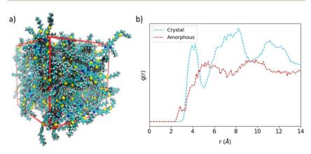
Fig. 8 (a) Representative snapshot of the amorphous IDIDF phase. (b) Radial distribution function (g(r)) of the centroid of a central molecule with respect to the other molecules in crystalline and amorphous IDIDF.
