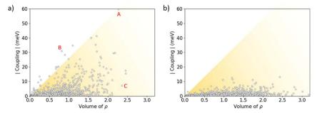
Fig. 9 Absolute value of the electronic coupling vs. the integrated volume of  $\rho$  associated to the weakly stabilizing non-covalent interactions for IDIDF (a) and spiro-OMeTAD (b) first-nearest dimers as obtained during the NPT molecular dynamics in the amorphous phase. The representation of the RDG index for representative dimers A, B and C of IDIDF is displayed in Fig. S9.†
