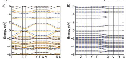
Fig. 6 Electronic band structures of (a) Ni-btt and (b) 100%-trans Ni-ibtt, calculated using the HSE06 functional. Spin-up bands are depicted by solid orange lines, spin-down by dashed blue lines, and the valence band maximum is set to 0 eV. This figure was plotted using the sumo package.<sup>33</sup>
