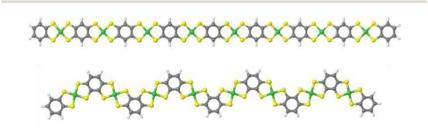
Fig. 4 Minimum energy conformations obtained from DFT calculations for octamers of Ni-btt (top) and Ni-ibtt (bottom) with all metal-ligand complexes in trans-configuration.
