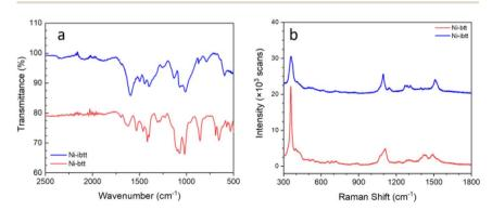
Fig. 3 FTIR (a) and resonance Raman (728 nm excitation) (b) spectra of Ni-btt and Ni-ibtt after purification. The spectra have been stacked for clarity.
