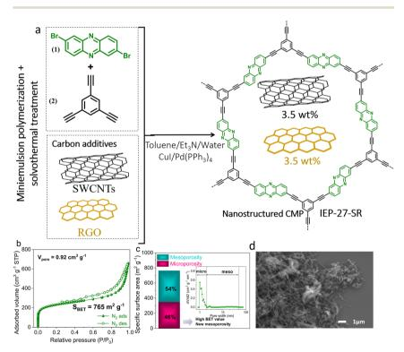
Fig. 1 (a) Synthesis scheme of the IEP-27-SR hybrid. (b) Nitrogen adsorption—desorption isotherm. (c) Percentages of micro-/mesoporosity and pore-size distribution of IEP-27-SR (inset) from the quenched solid density functional theory (QSDFT) model. (d) FE-SEM image of the IEP-27-SR hybrid. The scale bar is 1 μm.
