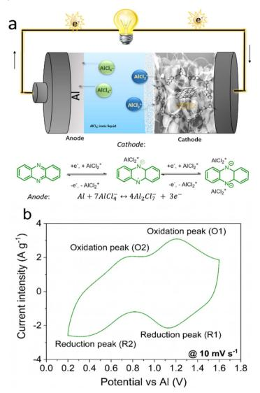
Fig. 2 (a) Scheme of the aluminium-phenazine battery during discharge and general redox working mechanism of the phenazine unit and Al reactions. (b) CV recorded at  $10~\text{mV}~\text{s}^{-1}$  illustrating the two sequential one-electron and one-AlCl<sub>2</sub>+ redox reaction steps.
