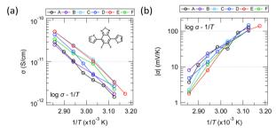
Fig. 10 Temperature dependence of the (a) electrical conductivities and (b) Seebeck coefficients of six molecules having the same molecular skeleton shape but different heteroatoms.
