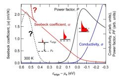
Fig. 1 Dependence of electrical conductivity and Seebeck coefficient in three-dimensional semiconductors on the chemical potential of electrons calculated using eqn (2) and (3).
