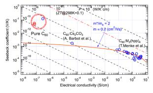
Fig. 2 Seebeck coefficient and electrical conductivity of pure and doped C<sub>60</sub> thin films measured at room temperature. The red curve indicates eqn (4) fitted to the results with doped C<sub>60</sub> films.<sup>11,12</sup> Red marks indicate positive Seebeck coefficients and blue ones negative.
