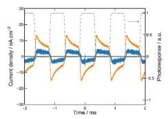
Fig. 4 Time trajectory of the transient photocurrent for the [ITO|I|S|I|Ag] photocell. The orange and blue curves show the photocurrent when S = ET-PRBT and EO-PRBT, respectively, and the gray broken curve indicates the response from a Si diode to monitor the light-on and -off periods.
