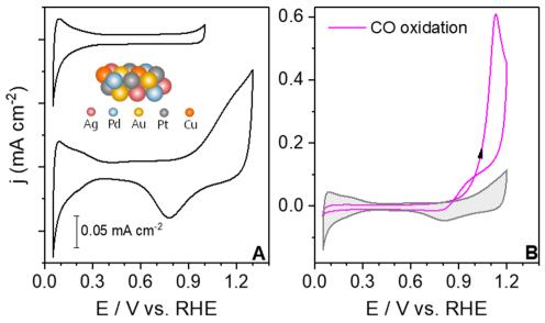
Fig. 1 (A) Blank cyclic voltammograms of an extended AgAuCuPdPt HEA in contact with  $0.1 \,\mathrm{M}$  HClO<sub>4</sub> saturated in an Ar atmosphere at 50 mV s<sup>-1</sup> at two different potential windows. (B) The magenta solid line corresponds to the CO oxidation curve in CO-saturated atmosphere at 50 mV s<sup>-1</sup> and the grey shadow to the blank cyclic voltammogram on the extended AgAuCuPdPt HEA.
