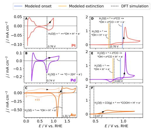
Fig. 2 Blank stable cyclic voltammograms of (A) Pt (poly), (B) Pd (poly), and (C) Au (poly) in contact with 0.1 M HClO<sub>4</sub> saturated in an Ar atmosphere at 50 mV s $^{-1}$  and (D)–(F) corresponding CO oxidation curves in CO-saturated atmosphere at 50 mV s $^{-1}$ . Equilibrium potentials obtained with DFT simulations (black dashed lines) as well as modelled equilibrium potentials for \*OH adsorption at low (vertical orange line) and high (vertical blue line) \*CO coverage are shown
