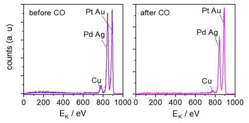
Fig. 4 ISS spectra of an extended AgAuCudPt. HEA before and after continuous CO oxidation, after five scans
