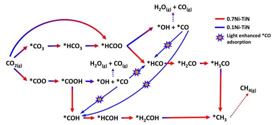
Proposed reaction mechanism over 0.7Ni-TiN and 0.1Ni-TiN
