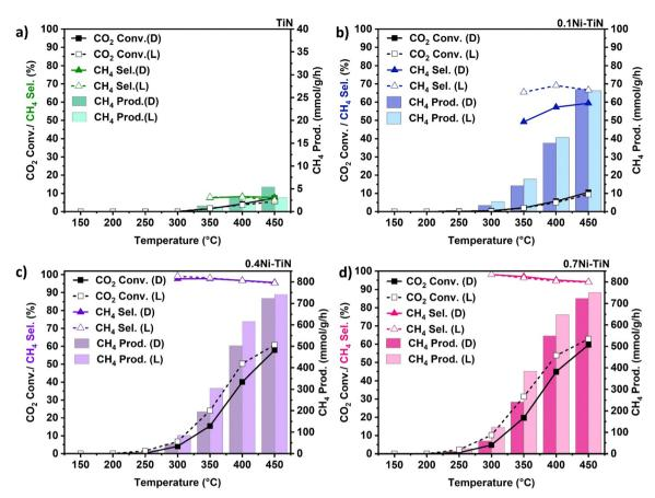
Fig. 3 CO<sub>2</sub> methanation reaction activity (conversion (Conv.), CH<sub>4</sub> production (Prod.)) and CH<sub>4</sub> selectivity (Sel.) with temperature over (a) neat TiN; (b) 0.1Ni-TiN, (c) 0.4Ni-TiN, and (d) 0.7Ni-TiN under non-illuminated (D) and illuminated (L) conditions conducted within a Harrick reactor (24 mL min<sup>-1</sup>, CO<sub>2</sub>: N<sub>2</sub>: H<sub>2</sub> = 1:1:4, 150 °C-450 °C).
