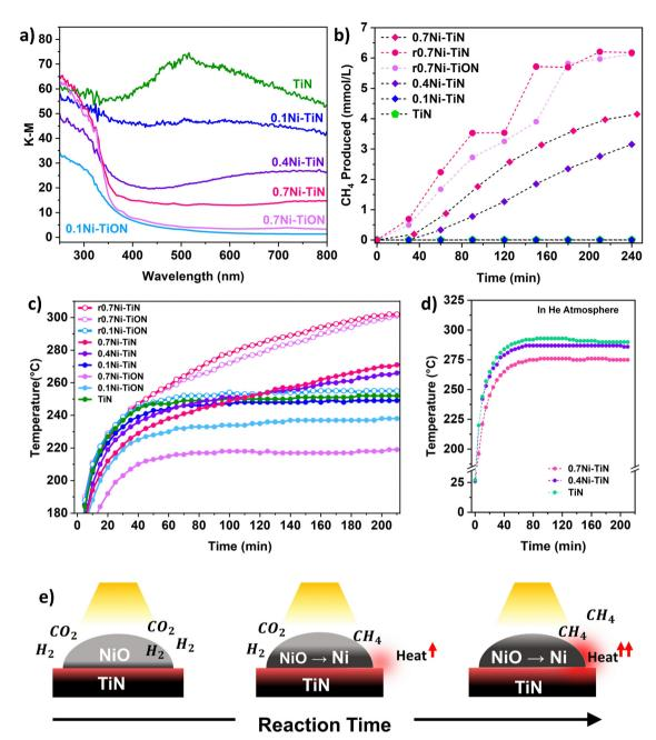
Fig. 2 (a) UV-vis absorption spectra for neat TiN, 0.1Ni-TiN, 0.4Ni-TiN, 0.7Ni-TiN and oxidised controls (0.1Ni-TiON, 0.7Ni-TiON); (b) photothermal CH<sub>4</sub> production by the various samples; (c) corresponding temperature profiles under photothermal conditions (Xe lamp at 20A setting); (d) xNi-TiN temperature profiles under inert He atmosphere (~80 kPa); (e) proposed photothermally-driven in situ Ni reduction mechanism.
