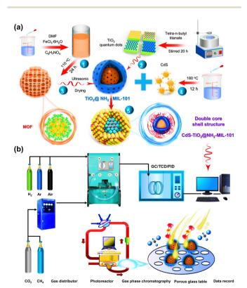
Scheme 1 (a) Schematic diagram of the process for preparing the ternary composites; (b) process flow equipment diagram for photocatalytic CH<sub>4</sub> dry reforming
