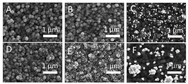
Fig. 5 SEM images of FTO/Au/Sb<sub>2</sub>Se<sub>3</sub>/TiO<sub>2</sub> with Au cocatalyst deposited at different biases -0.4 V (left: A and D), -0.25 V (middle: B and E), and 0.1 V (right: C and F) [referenced vs. Ag/AgCl] and at varying amounts of charge passed in mC cm<sup>-2</sup>: 25 (top: A-C), 75 (bottom: D-F). The scale bar corresponds to 1 µm.
