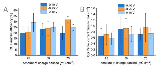
Fig. 7 (A) Faradaic efficiency for CO of the FTO/Au/Sb<sub>2</sub>Se<sub>3</sub>/TiO<sub>2</sub>/Au photoelectrode with corresponding (B) partial current density for CO at different deposition bias (-0.4 V, -0.25 V, 0.1 V vs. Ag/AgCl) and different amount of charge passed (25, 50, 75 mC cm<sup>-2</sup>) for the Au catalyst deposition.
