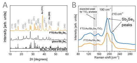
Fig. 2 (A) XRD patterns of Sb<sub>2</sub>Se<sub>3</sub> thin films prepared on glass and FTO/Au. (B) Raman spectra of FTO/Au/Sb<sub>2</sub>Se<sub>3</sub> films before and after TiO<sub>2</sub> deposition.
