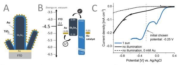
Fig. 4 (A) Schematic representation of the photoelectrode assembly with the corresponding (B) band diagram. (C) Linear sweep voltammogram of the photoelectrode with and without 1 sun illumination with UV filter (AM1.5G, 100 mW cm<sup>-2</sup>,  $\lambda > 400$  nm) in a solution of 0.5 mM KAuCl<sub>4</sub> and 0.25 mM H<sub>2</sub>SO<sub>4</sub> with 5% v/v methanol.
