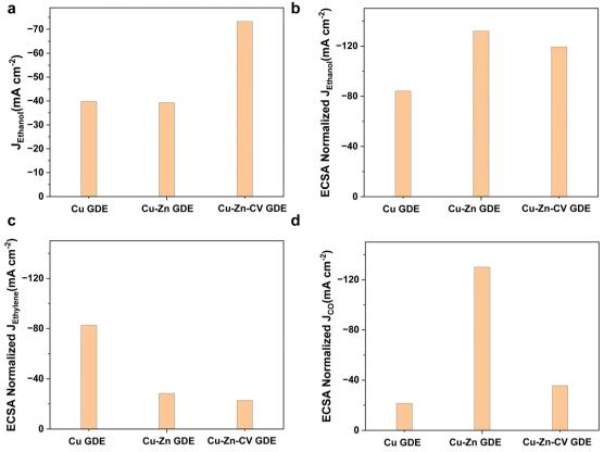
Fig. 6 Cu-GDE, Cu-Zn-GDE and Cu-Zn-CV-GDE three electrodes at a current density of -250 mA cm<sup>-2</sup>. (a) Partial current density of ethanol production. ECSA normalized partial current densities of (b) ethanol, (c) ethylene, and (d) carbon monoxide.
