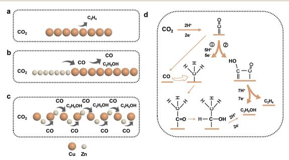
Fig. 7 Proposed mechanism of ethanol formation over (a) Cu-GDE, (b) Cu-Zn-GDE and (c) Cu-Zn-CV-GDE catalysts, and (d) the main product of ethanol and ethylene formation during CO<sub>2</sub> reduction electron transfer and proton coupling steps.
