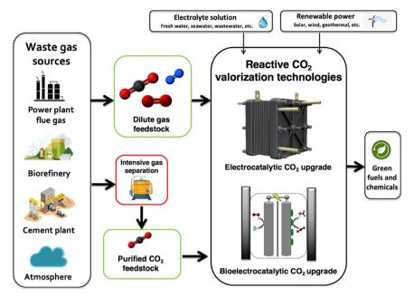
Fig. 1 Overview of emerging CO<sub>2</sub> capture and conversion pathways. Proposed process flow for electrified CO<sub>2</sub> conversion with selection of waste gas feedstock, omission or inclusion of gas separation device, and choice of CO<sub>2</sub> conversion nanotechnology.
