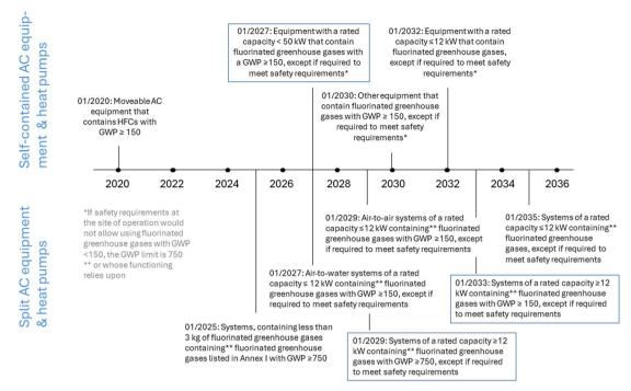
Fig. 3 Placing-on-the-market prohibitions from Annex IV of the F-gas Regulation9 that refer to self-contained air conditioning (AC) equipment and heat pumps, except chillers (upper part), and split AC equipment and heat pumps (lower part). The blue boxes indicate systems with a rated capacity ≥12 kW.
