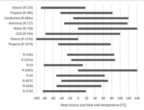
Fig. 1 Application range of some of the fluorinated and some of the non-fluorinated refrigerants. The lower limit is the normal boiling point, the upper limit is the temperature 15 °C below the substance's critical temperature. Exceptions are R-744 and R-718. Graphic is cut at -100 °C and 140 °C. Adapted from IEA [2020].<sup>39</sup>
