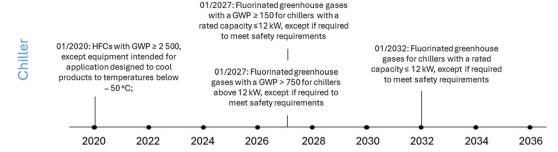
Fig. 4 Placing-on-the-market prohibitions from Annex IV of the F-gas Regulation<sup>9</sup> that refer to chillers
