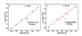
Fig. 4 Model of CI for microplastic PE with different particle sizes during the weathering process, (a) PE-30; (b) PE-125.
