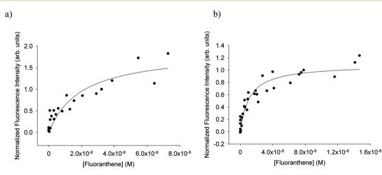
Fig. 3 Normalized isotherms for (a) fluoranthene in freshwater and (b) fluoranthene in 6 mM octanol from all successful experiments. The fits shown are those for all of the normalized isotherms combined. The correlation coefficients and b values are: (a)  $b = (1.97 \pm 0.70) \times 10^{-8}$ ,  $r^2 = 0.70$ 0.83; (b)  $b = (1.12 \pm 0.23) \times 10^{-9}$ ,  $r^2 = 0.90$ .
