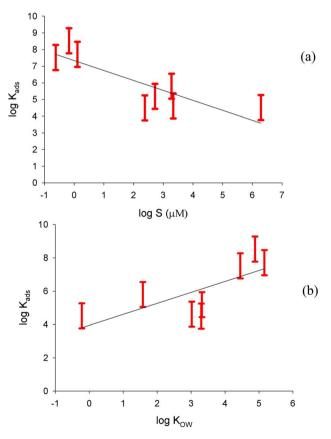
Fig. 4 Plots of  $\log K_{ads}$  as determined here against (a)  $\log S$ , with the solubility expressed in  $\mu$ mol L<sup>-1</sup>; (b) log  $K_{OW}$ . The red bars indicate the range of  $\log K_{ads}$  values calculated with different assumptions of the maximum surface coverage, including experimental uncertainties. The black lines show a linear regression, representing an LFER.
