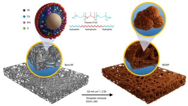
Fig. 1 Schematic representation of the fabrication process for the NCMP electrode. Schematic illustration of the one-pot and constant current (-10 mA cm<sup>-2</sup>, 2.5 h) electrosynthesis of the NCMP film on a nickel foam substrate. The chemical structure, amphiphilic character, and the possible morphological transition of Pluronic P123 in aqueous electrolyte, which results in a morphology-controlled electrocatalyst film, is also presented.
