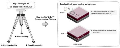
Scheme 1 Schematic representation of the manganese oxide cathode based on a dual-ion co-intercalation strategy that simultaneously boosts surface Mn<sup>2+</sup>/Mn<sup>4+</sup> two-electron transfer and maintains the stability of the host material structure to cope with the key challenges of mass loading, cycling stability, and specific capacity in Mn-based cathodes.
