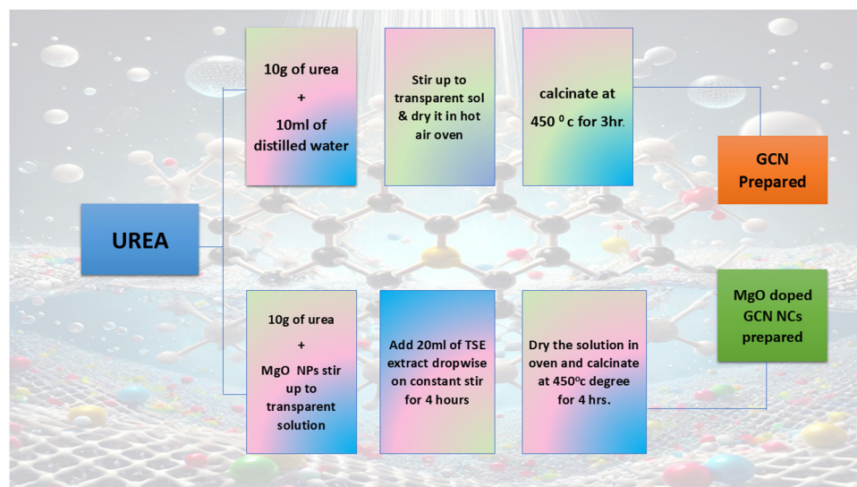
Fig. 3 Fabrication of MgO doped g-C 3 N 4 nanocomposites (MgCN) at varying conc.
