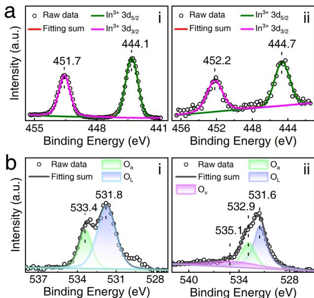
Fig. 2 Chemical state analysis. (a) In 3d XPS spectra of (i)  $\text{In}_2\text{O}_3$  and (ii) Pd/ $\text{In}_2\text{O}_3$ . (b) O 1s XPS spectra of (i)  $\text{In}_2\text{O}_3$  and (ii) Pd/ $\text{In}_2\text{O}_3$ .
