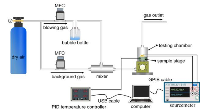
Scheme 2 Schematic diagram of the gas-sensing measurement system.
