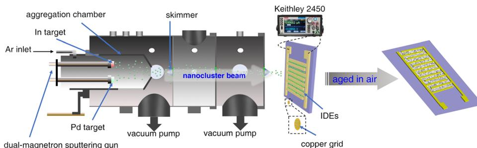
**Scheme 1** Schematic diagram of the fabrication of the ethanol vapor sensor device based on Pd/In<sub>2</sub>O<sub>3</sub> hybrid NCs.
