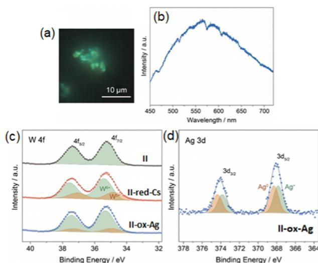
Fig. 10 PL (a) image and (b) spectrum of **II-ox-Ag** with excitation at 405 nm. Narrow scan XPS spectra (c) W 4f and (d) Ag 3d of with deconvolution. Reprinted with permission from Haraguchi *et al.* Copyright 2021 Wiley-VCH.
