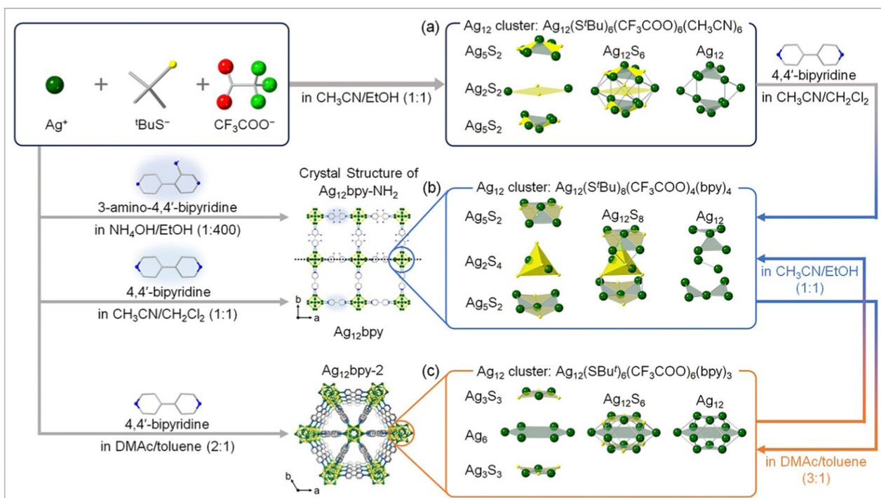
Fig. 1 Design approach and schematic illustration of the syntheses and structures of **Ag**<sub>12</sub>-based SCC-MOFs. (a) **Ag**<sub>12</sub>, (b) **Ag**<sub>12</sub>**bpy** and **Ag**<sub>12</sub>**bpy-NH**<sub>2</sub>, and (c) **Ag**<sub>12</sub>**bpy-2**.
