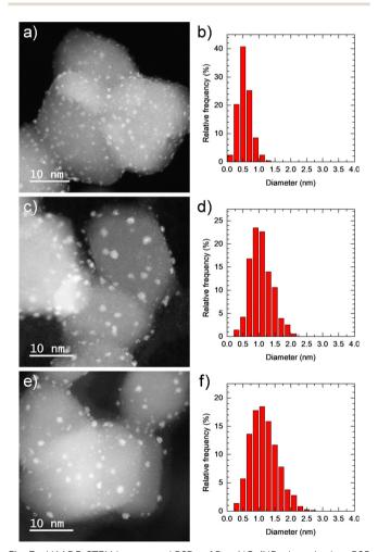
Fig. 3 HAADF-STEM images and PSDs of Pt s-NCs/NPs deposited on P25 TiO<sub>2</sub> surface at room temperature (i.e., 25 °C) after 5 ALD cycles (a) and (b), followed by the annealing in air at 400  $^{\circ}$ C for 3 h (c) and (d) and 6 h (e) and (f).
