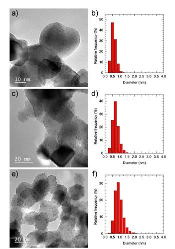
Fig. 2 TEM images and PSDs of Pt NPs deposited on P25  $TiO_2$  surface at 100 °C after 1 cycle (a) and (b), 5 cycles (c) and (d) and 10 cycles (e) and (f).
