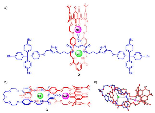
Fig. 4 Knighton and Beer's heteroditopic (a) [2]rotaxane 2 and (b) [2]catenane 3, based on interlocked calix[4]diquinone and pyridine-N-oxide components. (c) Single crystal XRD structure of [2]catenane bound to an NaCl ion-pair.
