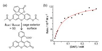
Fig. 3 (a)  $\mathbf{H}^{\mathbf{w}}$ -catalysed hydrolysis of diacetyl fluorescein; (b) dependence of the reaction rate on substrate concentration, fitted to a Michaelis Menten reaction model to extract an association constant for the interaction between substrate and cage exterior surface (see main text).
