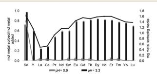
Fig. 17 Sorption at pH 0.9 and 3.3 using  $\bf 39$ . Reprinted with permissions from Hovey  $\it et al., ^{124}$  copyright 2021, with permission from Elsevier.
