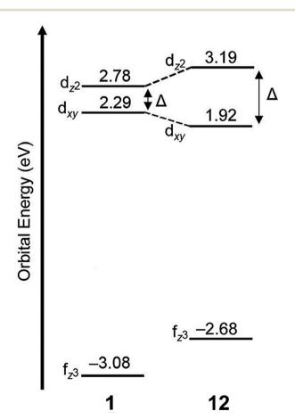
Fig. 8 Calculated d-orbital splitting of Eu<sup>II</sup>1 and Eu<sup>II</sup>12. Adapted from Corbin et al., 81 copyright 2018, with permission from Elsevier.
