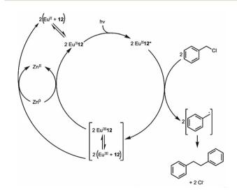
Fig. 12 Proposed photoredox catalytic mechanism of Eu<sup>II</sup>12 for reductive coupling reactions of benzyl chloride
