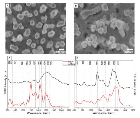
Fig. 3 SEM images of Aq-coated silicon nanopillar substrates (A) before and (B) after their leaning mode due to the drying process. Averaged SERS spectra of artificial (black) and liquid (red) cerumen absorbed, respectively, on (C) Ag-coated and (D) Au-coated SERS substrates. Spectral range: 600-2000 cm<sup>-1</sup>. Spectra are offset for clarity.
