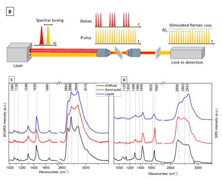
Fig. 4 Schematic illustrations of (A) the home-built BCARS and (B) SRS setups. Averaged (C) BCARS and (D) SRS spectra of artificial (black), semisolid (red) and liquid (blue) cerumen. Wavenumber range between 900 and 3200 cm<sup>-1</sup>. The spectra are cut in the silent region between 1800 and 2750 cm<sup>-1</sup>. Spectra are offset for clarity
