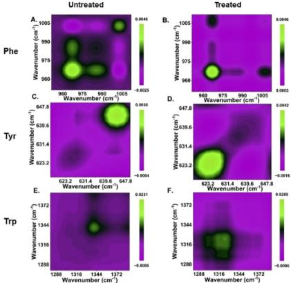
Fig. 4 Two-dimensional synchronous correlation map of untreated and treated cells. (A and B) phenylalanine; (C and D) tyrosine; (E and F) tryptophan. Each map includes the mean Raman spectra of different incubation time points to provide the spectral dynamics over the perturbation range. The green signal represent positive while magenta signal represent negative.
