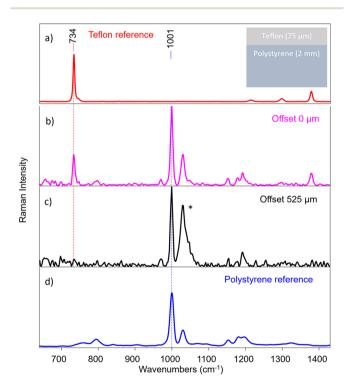
(a) Reference spectrum of pure Teflon; (b) spectrum of the first pair of fibres from S1 (Teflon over polystyrene) micro-SORS series; (c) spectrum of the last pair of fibres of the same series; (\*) the increase of highlighted peak is induced by an artefact; (d) reference spectrum of pure polystyrene. The instrument provides efficient surface to substrate contrast, as the characteristic peak of Teflon disappears.
