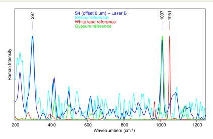
Fig. 11 Offset 0 spectrum of S4 analysed with the system coupled with Laser B, compared with the reference spectra of the Sienna pigment (top layer), white lead (bottom layer) and gypsum (preparation layer). The main band of Sienna pigment is clearly visible (297 cm<sup>-1</sup>), along with the gypsum band at 1007 cm<sup>-1</sup>. No white lead signal can be seen.
