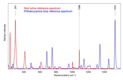
Fig. 7 Reference spectra of the two painted layers of S2, directly acquired on parts of the sample where they are not overlapped. The reference frequencies for each compound are indicated: 291 cm<sup>-1</sup> for red ochre, 1086 cm<sup>-1</sup> for calcite and 1531 cm<sup>-1</sup> for phthalocyanine blue.
