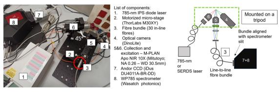
Fig. 2 Photo (a) and schematics (b) of the prototype with each component labelled.
