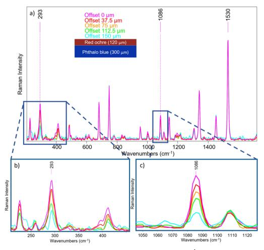
Fig. 8 (a) Micro-SORS measurement of S2 where all spectra have been normalized to the 1530 cm<sup>-1</sup> band of the bottom layer. The SORS effect is clearly visible for raman bands of (b) red ochre and (c) calcite.
