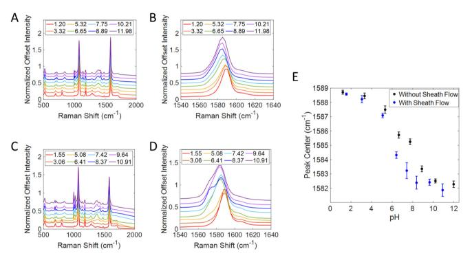
Fig. 3 SERS spectra of MBA while flowing PBS solutions over the surface at varying pH values with sheath flow off (A) with a zoom in on the 1585 cm $^{-1}$  band (B), and with sheath flow on (C & D). The center of the 1585 cm $^{-1}$  band was used to create a titration curve (E). The inflection point on this curve is much sharper when the sheath flow was on.
