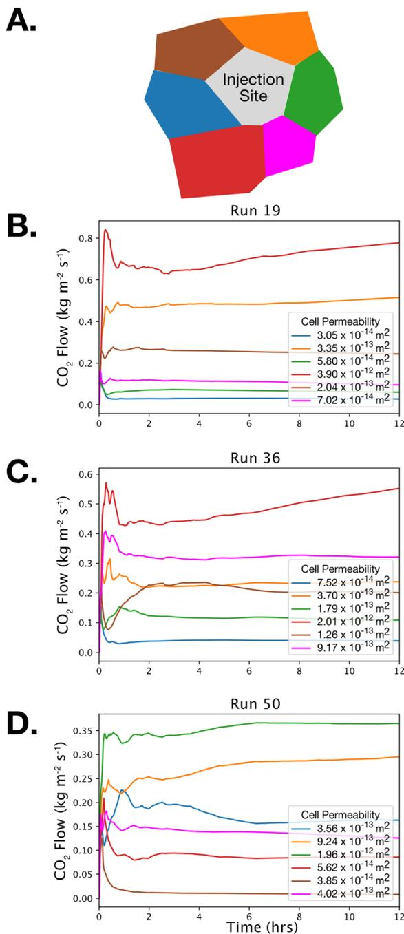
**Fig. 8** Simulation results of CO<sub>2</sub> flow rate from one injection cell into adjacent grid cells for ensemble simulations 19, 36, and 50 in early time. Panel A illustrates the spatial configuration of grid cells adjacent to the injection cell. Color codes are repeated in cells B–D, which illustrate the CO<sub>2</sub> flow rate (kg m<sup>-2</sup> s<sup>-1</sup>). Note that high permeability grid cells receive higher CO<sub>2</sub> flow rates.
