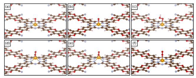
Fig. 4 Examples of the structure of (a) OH\*, (b) O\*, (c) OOH\*, (d) OH\*OH\*, (e) OH\*O\*, and (f)  $O_2$ \* intermediates on COF-based SACs.
