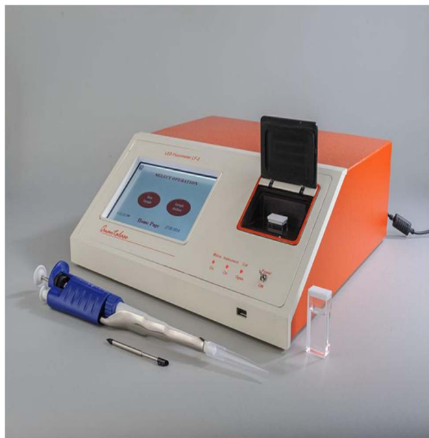
Fig. 2 LED fluorimeter (model LF-2) (QUANTALASE, India).
