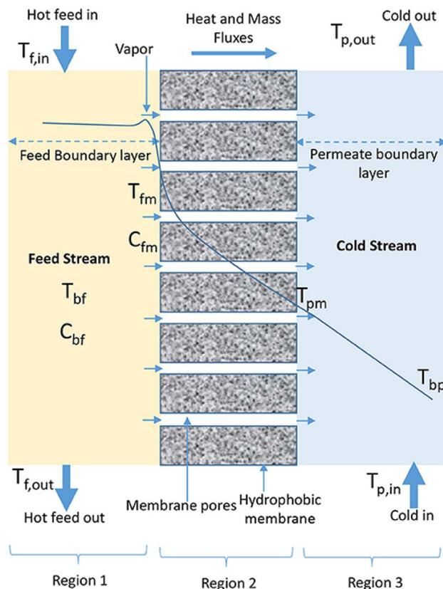
Fig. 4 Temperature polarization phenomenon in MD.  $T_{f,in}$ ,  $T_{fm}$ ,  $T_{pm}$  and  $T_{pb}$  represent temperatures in the bulk feed solution, near the membrane surface (feed side), near the membrane surface (permeate side) and in the bulk permeate, respectively.<sup>58</sup>
