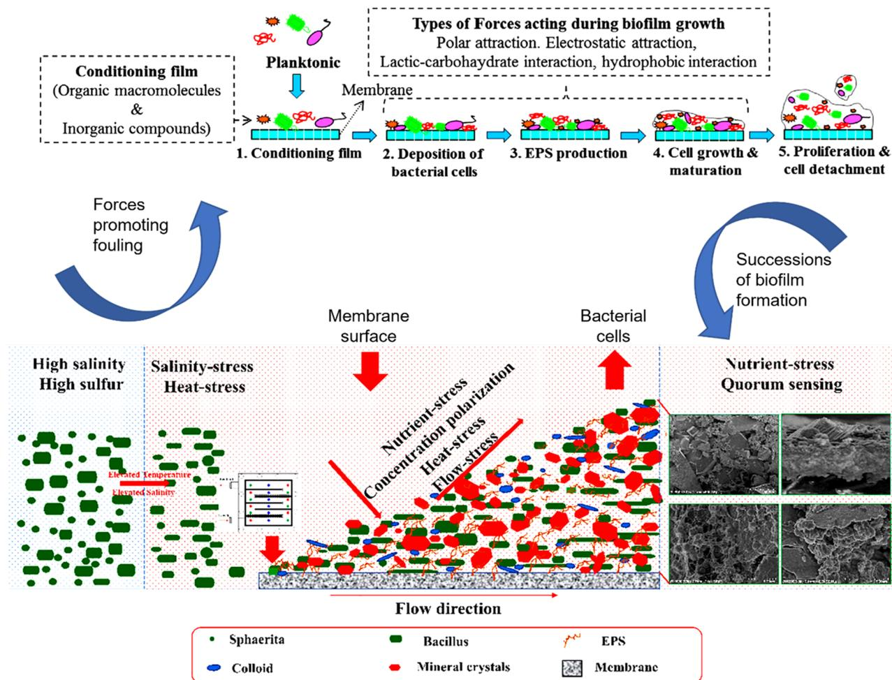
Fig. 2 Mechanistic relationship of the salinity, heat, nutrient, and flow stresses on the distribution of bacteria on membrane surfaces during MD operation.<sup>30,32</sup>
