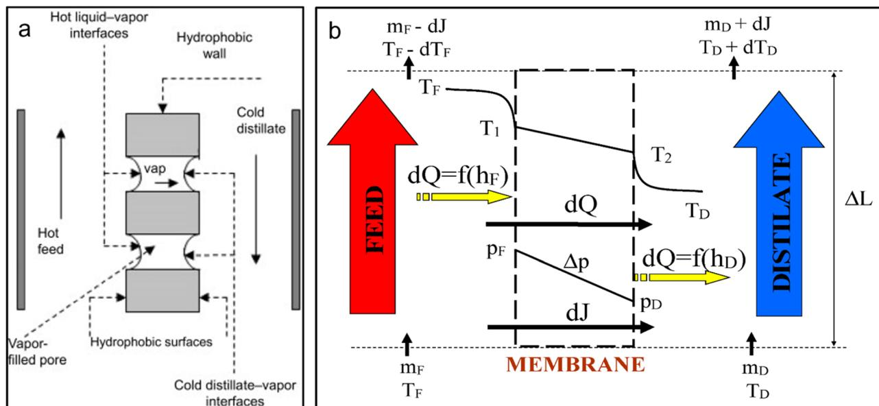
Fig. 1 Mechanism of operation of MD: (a) process mechanism and (b) heat and mass transfer, where  $T_F$ ,  $T_D$ ,  $T_1$ ,  $T_2$ ,  $P_F$ ,  $P_D$ ,  $\Delta p$ ,  $dQ$  represent feed, distillate, evaporation and condensation temperatures, feed and distillate vapour pressure, vapor partial pressure difference and change in energy respectively.<sup>13–15</sup>
