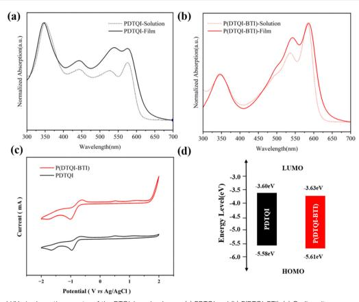
Fig. 3 Normalized UV-vis absorption spectra of the DTQI-based polymers (a) PDTQI and (b) P(DTQI-BTI). (c) Cyclic voltammograms of polymer thin films measured in 0.1 M tetrabutylammonium hexafluorophosphate acetonitrile solution with the Fc/Fc+ redox couple as an external standard at a scanning rate of 0.05 V s<sup>-1</sup>. (d) FMO level diagram of the DTQI-based polymer films.
