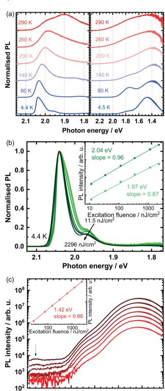
Fig. 2 (a) Temperature-dependent photoluminescence spectra of OBESnl<sub>4</sub> (left panel) and EDBESnI<sub>4</sub> (right panel). Power-dependent photoluminescence spectra at 4.4 K of (b)  $OBESnI_4$  and (c)  $EDBESnI_4$ , where the insets show the doublelogarithmic plots of the photoluminescence intensity versus excitation fluence.
