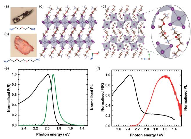
Fig. 1 (a) OBESnI<sub>4</sub> and (b) EDBESnI<sub>4</sub> images of mm-sized single crystals. Crystal structure of (c) OBESnI<sub>4</sub> and (d) EDBESnI<sub>4</sub>, where grey atoms are Sn, purple are I, blue are N, brown are C, red are O, and white are H. The inset highlights the formed hydrogen bonds. Kubelka–Munk transformed diffuse reflectance and photoluminescence spectra of (e) OBESnI<sub>4</sub> and (f) EDBESnI<sub>4</sub>.
