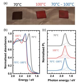
Fig. 3 (a) Optical image of OBESnI $_4$  thin films processed at 70 °C, 100 °C, and 70–100 °C. (b) Absorbance spectra and (c) photoluminescence spectra of the thin films.
