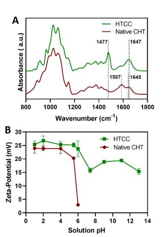
Fig. 4 (A) ATR-FTIR spectra of HTCC and native CHT powders. (B) Evolution of the  $\zeta$ -potential for 0.1 mg mL $^{-1}$  HTCC and CHT aqueous solutions as a function of the solution pH presented as mean  $\pm$  SD of three independent experiments (n=3, per condition) performed in triplicates.
