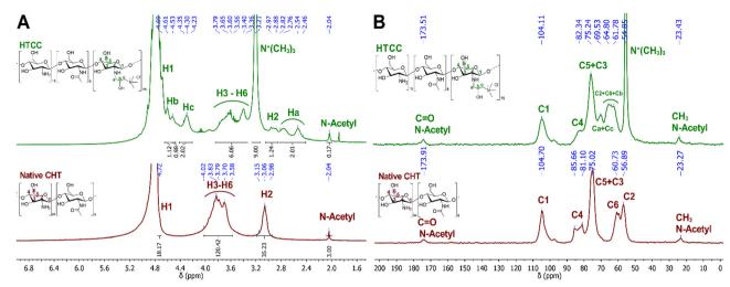
Fig. 3 (A)  $^1$ H NMR and (B)  $^{13}$ C NMR spectra of HTCC and native CHT biopolymers.
