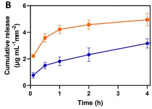
Fig. 9 (A) Cumulative mass release profile of FITC-BSA in PBS at pH 7.4 from (HTCC/ALG/HTCC/FITC-BSA)100 (blue line and circles) and (HTCC/ ALG)<sub>200</sub>/HTCC/FITC-BSA (orange line and squares) FS membranes over 96 h. (B) Zoom-in on the cumulative release of FITC-BSA for the first 4 h (represented with a dotted line in A). Data are presented as mean  $\pm$  SD of three independent experiments (n = 3, per condition) performed in triplicates.
