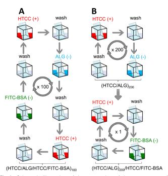
Fig. 1 Schematic illustration of the preparation of the two set-ups of FS multilayered membranes: (A) (HTCC/ALG/HTCC/FITC-BSA)<sub>100</sub> and (B) (HTCC/ALG)<sub>200</sub>/HTCC/FITC-BSA assembled onto poly(vinyl carbonate) substrates by resorting to attractive electrostatic interactions between HTCC, ALG and FITC-BSA.
