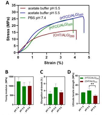
Fig. 8 Mechanical properties of the FS membranes in PBS (pH 7.4) and acetate buffer (pH 5.5). (A) Representative stress-strain curves, (B) Young modulus, (C) elongation-at-break, and (D) ultimate tensile strength. Data are presented as mean  $\pm$  SD of three independent experiments (n = 3, per condition) performed in triplicates. Significant differences were found for \*\*  $p \leq 0.01$ .
