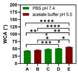
Fig. 7 WCA of all FS membrane formulations in PBS (pH 7.4) and acetate buffer (pH 5.5): (A) (HTCC/ALG/HTCC/FITC-BSA)<sub>100</sub>, (B) (HTCC/ALG)<sub>200</sub>, (C) (HTCC/ALG)<sub>200</sub>/HTCC/FITC-BSA, (D) (HTCC/ALG)<sub>200</sub>, and (E) (CHT/ALG)<sub>200</sub>. Data are presented as mean  $\pm$  SD of three independent experiments (n=3, per condition) performed in triplicates. Significant differences were found for \*\*\*\*  $p\leq 0.0001$ , \*\*\*  $p\leq 0.001$ , and \*  $p\leq 0.05$ .
