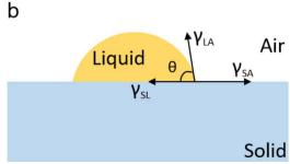
Fig. 1 (a) A schematic illustration of the interfacial absorbed NP, where R is the radius of NP. (b) Schematic illustration of a sessile droplet on a solid surface, with the relationship between the CA and surface tension  $\gamma$ . Reproduced with permission. <sup>22</sup> Copyright © 2019 Wiley-VCH GmbH.
