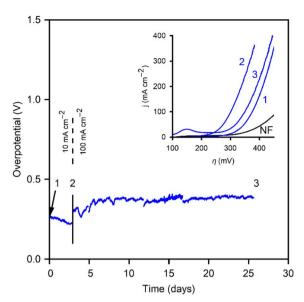
Fig. 9 CP curves of a CoNF electrode for  $10 \text{ mA cm}^{-2}$  (up to the black line) and 100 mA cm<sup>-2</sup>. Numbered points where the LSVs are taken are noted. Inset: polarization curves for the bare ANF and the three CoANF points noted in the CP curves.
