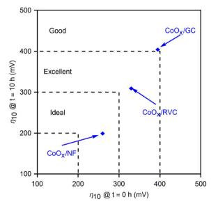
Fig. 10 Parametric plot of the overpotentials at a current density of 10 mA cm<sup>-2</sup> at the start of polarization (x-axis) and at t = 10 h (y-axis) for three CoO<sub>x</sub> films deposited on the three substrates: GC, RVC and NF, as well as the shaded regions representing where the (Ni/Co/FeO<sub>x</sub>) films deposited on different substrates fall. The dashed lines catalogue different activity regions into qualitative terms. All reported values are for the OER performed in 1.0 M KOH.
