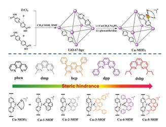
Fig. 1 Schematic view of the synthetic process (up) and the structures (down) of Cu-MOFs.
