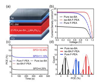
Fig. 4 (a) Device architecture of our Q-2D PSCs. (b) J-V curves, (c) steady-state PCEs at the maximum power point, (d) PCE histograms for 20 devices of pure iso-BA, iso-BA;F-PEA and pure F-PEA based PSCs.
