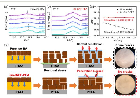
Fig. 2 GIXRD patterns at different instrument tilt angles for (a) pure iso-BA and (b) iso-BA:F-PEA based perovskite films. (c) Linear fit of  $2\theta$ -sin<sup>2</sup>( $\Psi$ ) of these two perovskite films. (d) Schematic illustration of strain relaxation, prevention of CB penetration through the perovskite film, and inhibition of re-dissolution of the PTAA layer via introducing the F-PEA SSC.
