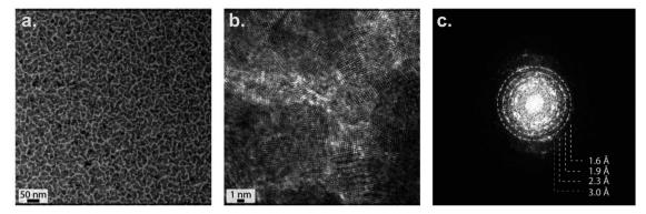
Fig. 8 Close interactions between Pd and CeO<sub>2</sub> are observed on TEM images with lighter areas corresponding to Pd rich domains while darker areas can be attributed to Ce-rich domains as shown on (a) and (b) TEM images and (c) FFT analysis.
