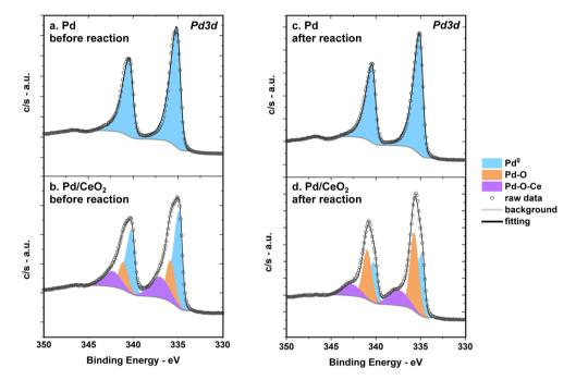
Fig. 9 XPS spectra measured before and after reaction show that Pd remains metallic on pure Pd thin films while Pd is partly oxidized on Pd/ CeO<sub>2</sub> as shown by the Pd 3d region of pure Pd (a) before reaction and (c) after reaction, and the Pd 3d region of Pd/CeO<sub>2</sub> (b) before reaction and (d) after reaction.
