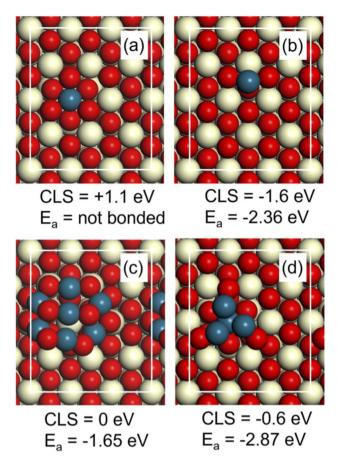
Fig. 10 The considered Pd-structures on  $CeO_2(111)$  have significant differences in Pd 3d core level shifts (CLS) and CO adsorption energy ( $E_a$ ). (a) Pd atom embedded in the top layer, (b) Pd atom adsorbed on the surface, (c)  $Pd_7O_8$  cluster, (d)  $Pd_4$  cluster with one atom embedded in the surface. The Pd 3d CLS are calculated with respect to PdO. Atomic color code: oxygen (red), palladium (blue) and cerium (beige).
