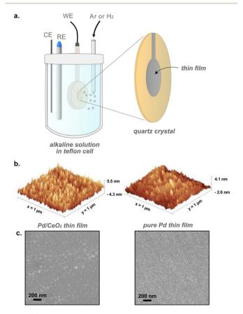
Fig. 1 (a) Schematic showing the setup used for *in situ* electrochemical characterization of thin films using E-QCM. RE, CE and WE refer to reference, counter and working electrodes, respectively. (b) Atomic force microscopy and (c) scanning electron microscopy images of Pd/CeO<sub>2</sub> and pure Pd thin films prepared by evaporation.
