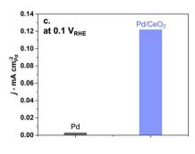
Fig. 2 The presence of  $CeO_2$  has a significant impact on hydrogen and oxygen interactions with Pd and leads to better HOR performance as shown in (a) CV at a 50 mV s<sup>-1</sup> scan rate in Ar-saturated 0.1 M KOH, (b) HOR performed in H<sub>2</sub>-saturated 0.1 M KOH at 5 mV s<sup>-1</sup> and 1600 rpm and (c) comparison of specific activity at 0.1 V<sub>RHE</sub> on pure Pd (black) and Pd/CeO<sub>2</sub> (blue).
