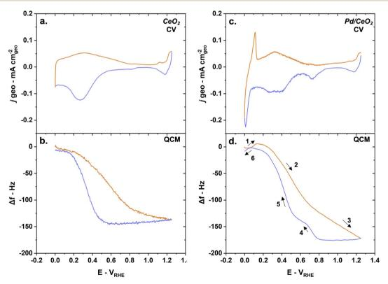
Fig. 5 The mass changes measured on Pd/CeO<sub>2</sub> are dominated by adsorption and desorption phenomena occurring on CeO<sub>2</sub> during conditioning as shown by (a) CV on CeO<sub>2</sub> and simultaneous (b) QCM measurements and (c) CV on Pd/CeO<sub>2</sub> and simultaneous (d) QCM measurements. The anodic scans are represented in orange while the cathodic scans are in blue. Reaction conditions: 5 mV s<sup>-1</sup> scan rate, Arsaturated 0.1 M KOH solution.
