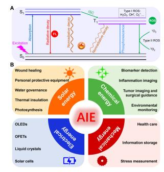
Fig. 1 (A) Jablonski diagram of different decay pathways of luminescent materials. (B) Scheme illustration of various energy conversion and applications based on AlEgens.
