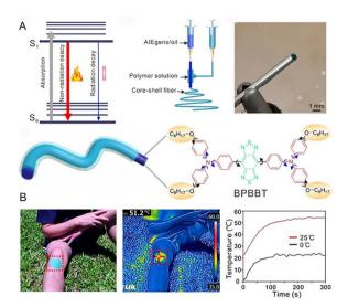
Fig. 6 (A) Jablonski diagram, setup of coaxial electrospinning, photograph of the core-shell needle, the structure of a core-shell fiber, and the molecular structure of BPBBT. (B) The optical and infrared images of a photothermal patch to warm the volunteer's knee in natural sunlight, and the temperature shift of BPBBT CS-3 at different ambient temperatures of 0 and 25 °C. Reproduced with permission from ref. 63. Copyright 2020, Wiley-VCH.
