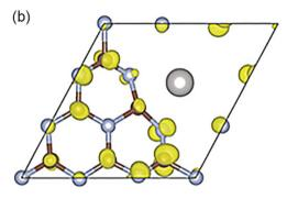
Fig. 2 (a) Energy-band alignment diagrams for  $q-C_3N_4$  and  $q-C_3N_4$ -Pt<sup>2+</sup>. (b) Photoexcited charge density transition from the Pt<sup>2+</sup>-induced hybrid highest occupied molecular orbital (HOMO) states to the lowest unoccupied molecular orbital (LUMO) of g-C<sub>3</sub>N<sub>4</sub>-Pt<sup>2+</sup>. Copyright 2016, Wiley-VCH.
