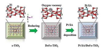
Fig. 1 The synthesis strategy for the Pt SA/Def-s-TiO<sub>2</sub> photocatalyst. Copyright 2021, Elsevier.
