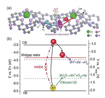
Fig. 7 (a) Schematic illustration of the solar-driven overall water splitting on the Co1-phosphide/PCN photocatalyst, in which the photogenerated electrons and holes (h<sup>+</sup>) are spatially separated. (b) Electronic band structure diagram for the Co1-phosphide/PCN photocatalyst. Copyright 2017, Wiley-VCH.
