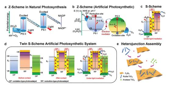
Fig. 12 Schematic illustration of (a) the Z-scheme in natural photosynthesis, (b) Z-scheme in an artificial photosynthetic system, (c) S-scheme, and (d) twin S-scheme artificial photosynthetic system before and after contact, and under illumination. (e) Schematic diagram of electrostatic self-assembly of material. Copyright 2022, Wiley-VCH.
