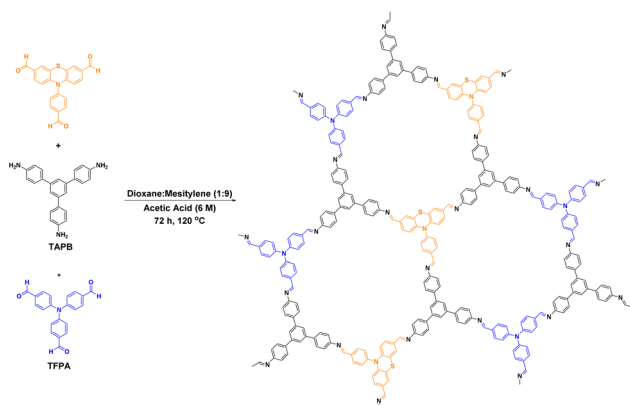
Fig. 12 Synthesis of a series of materials with different TFPA/3 molar ratios.
