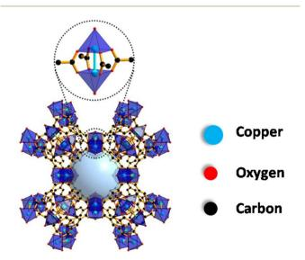
Fig. 1 Structure of HKUST-1 MOF. Reproduced from ref. 20.
