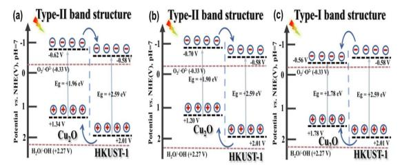
Fig. 3 The energy level illustration of (a) cubic, (b) truncated octahedral and (c) octahedral Cu<sub>2</sub>O@HKUST-1. Reproduced from ref. 25.
