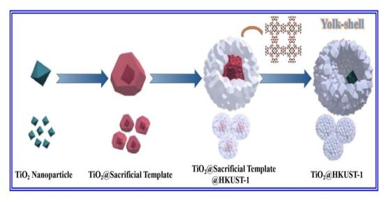
Schematic exhibition for the fabrication of TiO<sub>2</sub>@HKUST-1. Reproduced from ref. 24.
