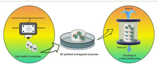
Fig. 3 3D printing of biocatalysts for flow biocatalysis.
