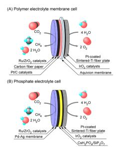
Fig. 1 Schematic illustration of polymer electrolyte membrane (A) and phosphate electrolyte (B) electrochemical cells for methane synthesis from CO<sub>2</sub> and H<sub>2</sub>O.
