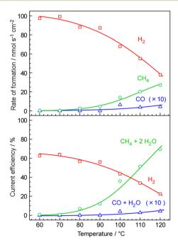
Fig. 2 Formation rates and the current efficiencies of CH<sub>4</sub>, H<sub>2</sub>, and CO as a function of temperature at 30 mA cm<sup>-2</sup> for the polymer electrolyte membrane cell with 10 wt%-Ru/ZrO<sub>2</sub>. The flow rate of CO<sub>2</sub> for the cathode vessel was 0.165 ml<sub>STP</sub> min<sup>-1</sup> and that of the mixture of Ar and H<sub>2</sub>O for the anode vessel was 10 ml<sub>STP</sub> min<sup>-1</sup> and 10  $\mu$ l<sub>Liquid</sub> min<sup>-1</sup>, respectively.
